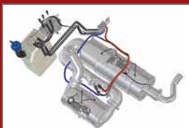
Tier 4 Final after-treatment package
