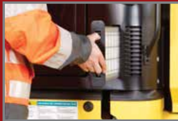
Interior cabin filter ease of access
