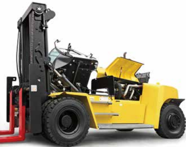
Powered cab tilt enables easy access to major components
