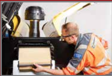
Gull wing hoods provide quick access
