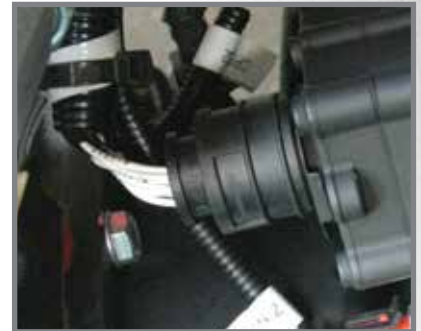
Standard profile Deutsch pin connectors, IP64 compliant
