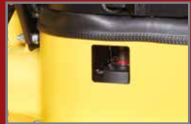
Hydraulic sight gauge for fluid level checks
